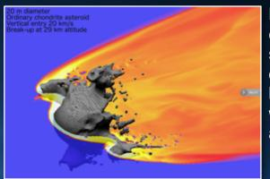
Researchers are running computational fluid dynamics simulations on Pleiades to determine the fragmentation and blast propagation that occurs when asteroids impact the atmosphere or the ground.
