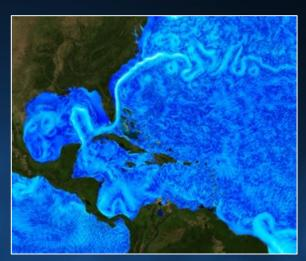
Researchers from the Estimating the Circulation and Climate of the Ocean (ECCO) consortium are running simulations on Pleiades to produce global, time-evolving maps of Earth's ocean and sea-ice system at an unprecedented resolution—about 1 kilometer (km) horizontal grid spacing.
