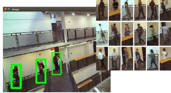
Detection uses OpenCV HOG descriptor and linear SVM. Detection size (window size) is (64, 128). The detector is written in Python and for 640x480 image, performs about 3 images/sec on current Waggle Edge processor.
