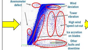
Predict wind energy of each turbine using manufacturer or empirical power curve algorithms
