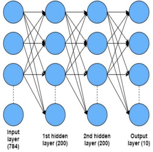
Fully connected neural network example architecture
